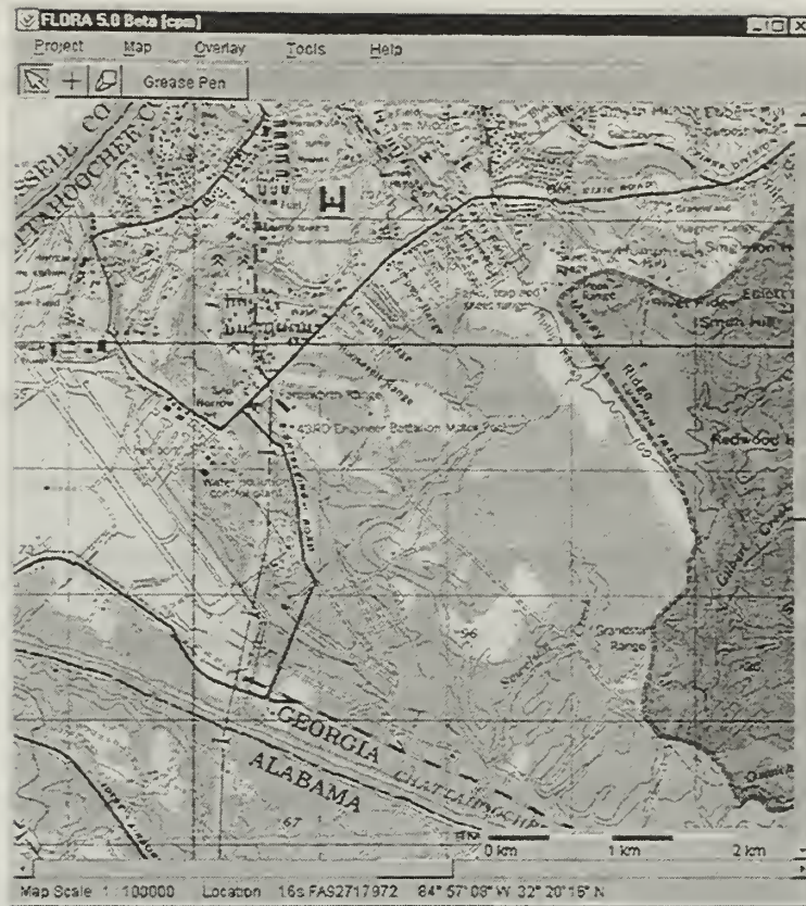
Figure 5. FLORA's map display was the first tool to include map annotation tools. The "Grease Pen" button launches a window with some basic annotation tools.
